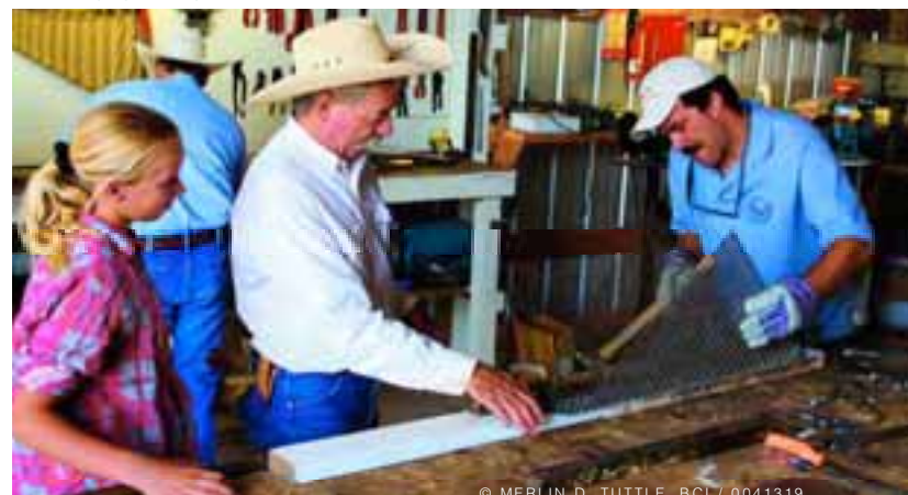
Dan Taylor (right) helps Dennis Maroney and his daughter, Allie, of the Cross-U Ranch in McNeal, Arizona, complete an expanded-metal escape structure by bending the sides to a 90-degree angle.
