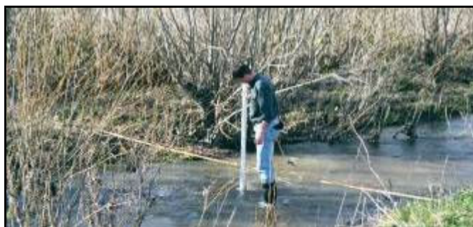
Figure 10: Tag Line measuring bankfull channel width and average depth for width:depth ratio.
