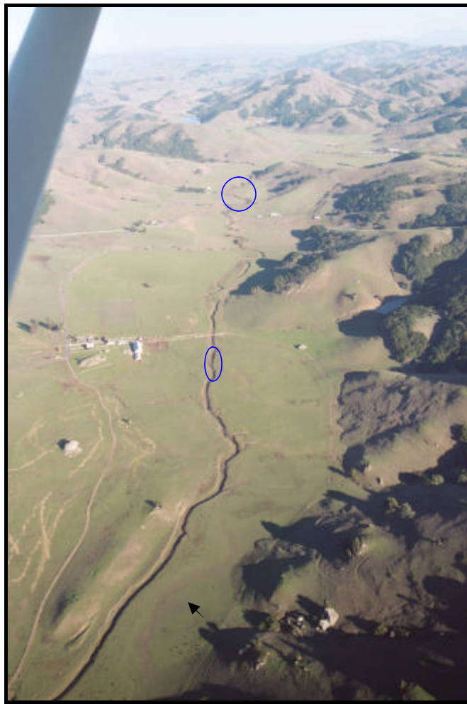
Figure 9. An example of the Alluvial Valley Transfer/Deposition Zone shown with Chileno Valley looking upstream. Straightened reach in lower left of photograph with black arrow pointing to possible original channel course. Blue circles indicate reference site locations.
