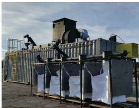
Pyrolysis System Rendering Pyrolysis converts biomass into carbon-sequestering biochar
