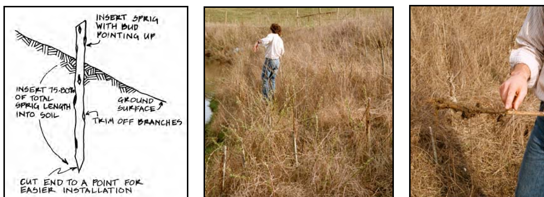
Figure 24: The specification for planting a willow cutting or sprig and surveying a newly planted site with some rabbit damage in 1988 (top). Design and photos by Prunuske Chatham, Inc.
