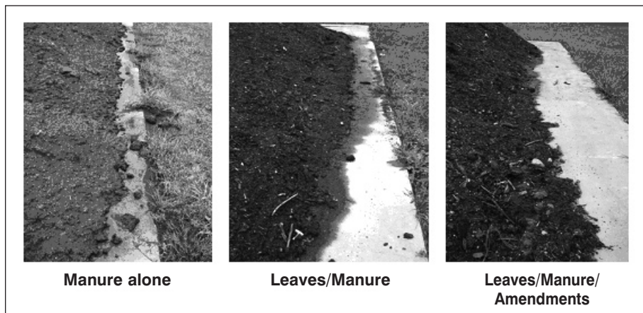
Figure 10. Surface leaching of pile nutrients and sediments after a heavy rain. The unmixed manure pile leached a greasy, smelly colloidal liquid (left), while the standard compost pile leached only a few odorless sediments (center), and the amended compost leached almost no water at all.
