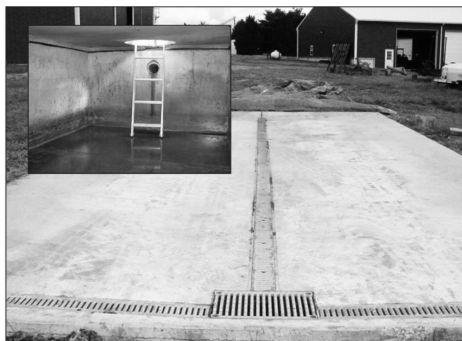
Figure 7. Compost pad with collection system. The inset picture shows the concrete pad on which the compost piles were constructed and aged. The drain grids in the middle and front of the pad collect water that runs through the compost pile and send it into a septic tank (the bottom picture, one tank for each pad) for later analysis.
