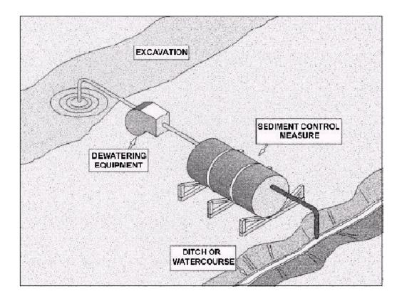
SEE ALSO; AQUA BARRIER STREAM BYPASS (WATER DIVERSION) COFFER DAM
