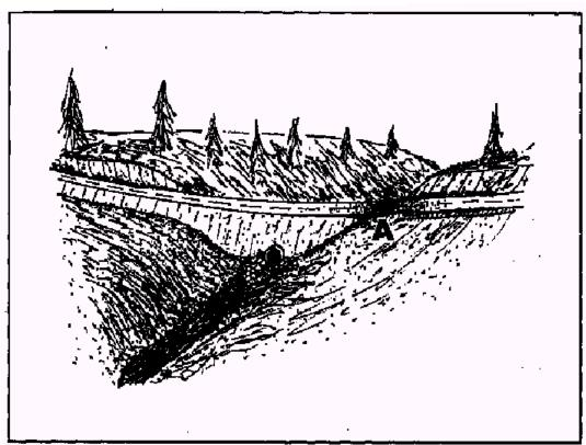
If culvert plugs, flow would reach the road surface and flow back into the channel at location "A" where the road changes grade.
