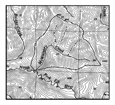
Figure 3.1 Drainage area calculation
