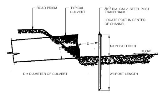
NOTE: THIS DESIGN KNOCKS BRANCHES AROUND POST TO PASS THROUGH CULVERT. FOR SMALL STREAMS ONLY.
