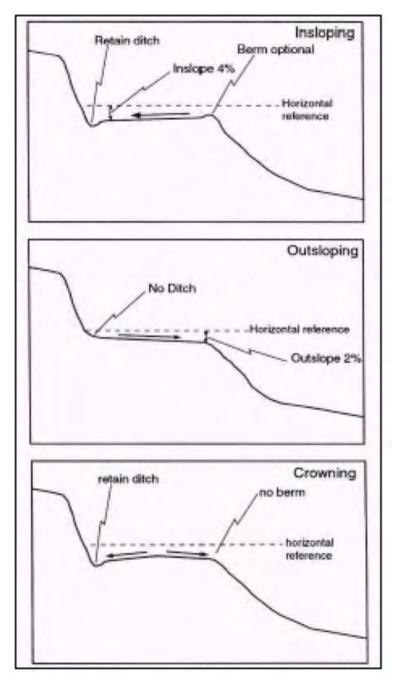
**Figure 5.3** Utilizing road shape to reduce surface runoff. California Salmonid Stream Habitat Restoration Manual Chapter X. CDFG 2002.
