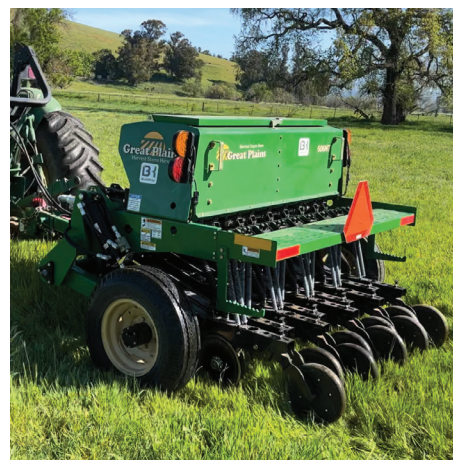
Marin RCD rents a no-till drill and seeder to small farmers to reduce soil erosion and nutrient runoff into nearby waterways.
